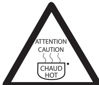
Avoid touching the cabinet surfaces which may have temperatures over 170° F. Use caution when opening either door due to steam exiting out.
